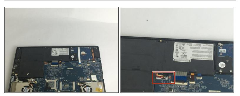
• After opening the bottom plate, locate the battery and the battery connection.
