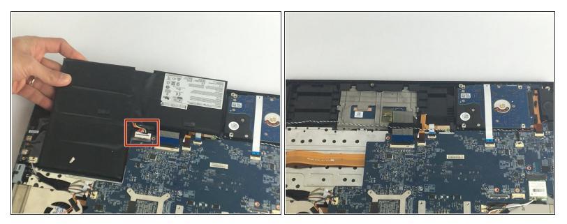
• Unplug the battery connection carefully from the motherboard, and remove the old battery.
