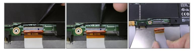
• The right ribbon cable has a <u>ZIF connector</u>. Use the flat end of your spudger to lift up the small locking flap, then pull out the cable.
