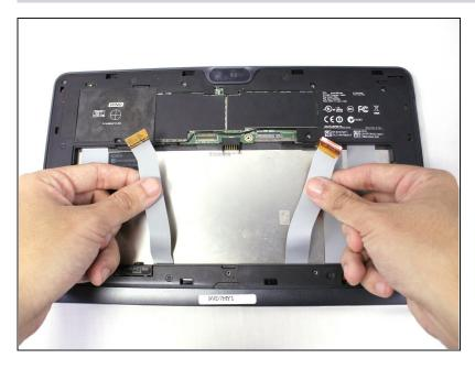
There are adhesive strips between the device and the two ribbon cables we disconnected. Pull each cable away from the device just enough to break the adhesive bonds.
