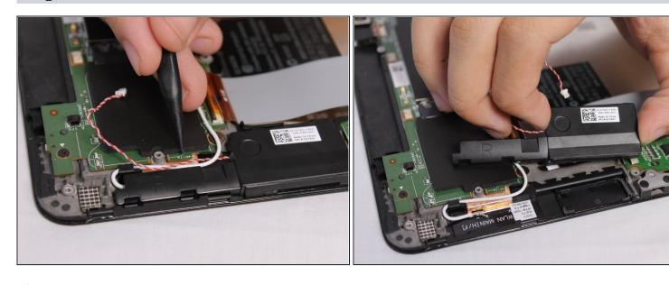
• Once the cable has been detached, use your fingers to lift the right speaker upwards to remove it.
