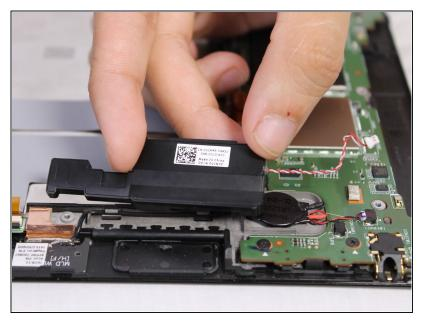
• Lift the right speaker upwards using your fingers to remove it.
