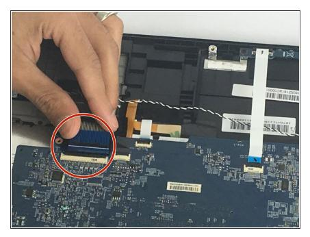
unplug the selected wire. Unplug it gently by lifting it up to unlock the black cover that connects it to the motherboard
