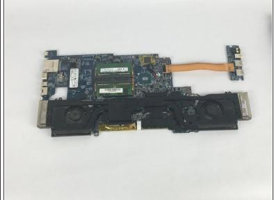
• After you remove all the connected wires and unscrew all the screws that holds the motherboard to the laptop, take the motherboard out as shown in the picture.
