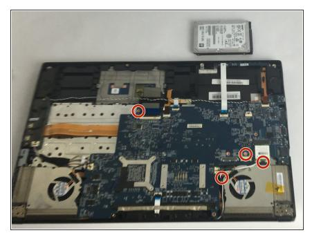
Remove the four 2.5mm screws with a PH0 bit.
