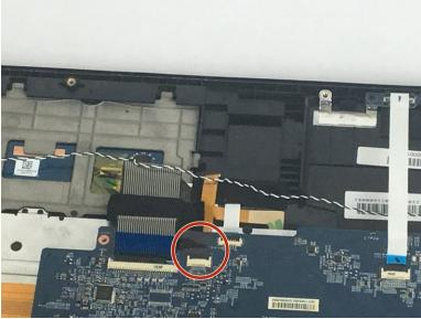
unplug the brown selected wire. Unplug it gently by lifting it up to unlock the black cover that connects it to the motherboard
