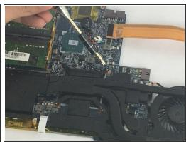
Remove the eight 2.5mm screws with a PH0 bit.
