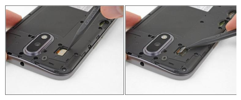
• Use a spudger to disconnect the camera flash connector by prying it straight up.
