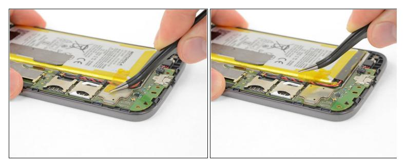
• Peel up and remove any tape connecting the battery to the main board.
