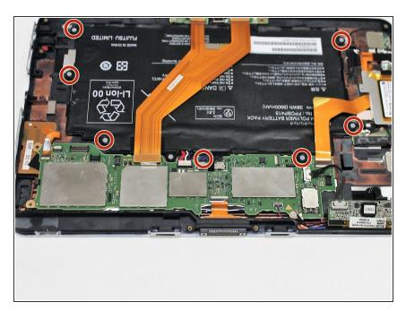
Remove seven 1mm screws using a PH00 screwdriver.
