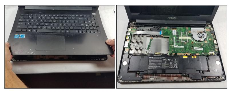
• Lift the keyboard assembly away from the remainder of the laptop.
