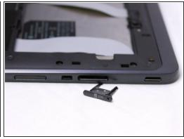
• Use your pin punch driver to push into the hole on the sim card, then pull out the sim tray.
