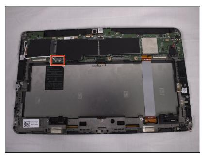
Next you must disconnect the black and white <u>coaxial</u> <u>connector cables</u>. We'll start with the black cable.
