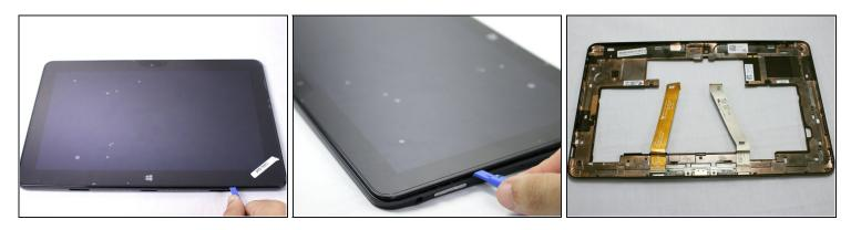
• Insert your plastic opening tool between the screen and frame, and run the tool around the edges to separate the frame from the tablet.
