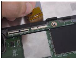
• Use the pointy end of your spudger to lift up the <u>ZIF</u> lock. Afterwards, pull the ribbon cable rearwards to disconnect it.
