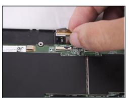
• To remove the left ribbon cable, use the pointy end of your spudger to flip the black **ZIF** retainer into the up position. Then simply pull it rearwards to remove it.
