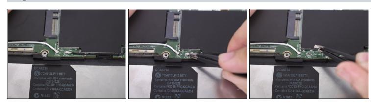
• Use the tweezers again to grab hold of the black <u>coaxial connector</u> and pull upwards to disconnect.
