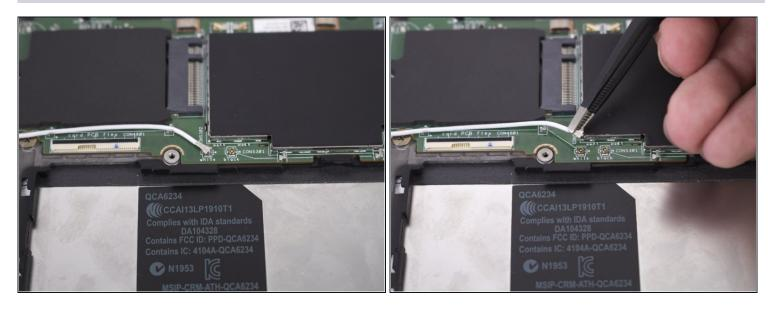
Now remove the white coaxial connector using the tweezers to pull the connector upwards.
