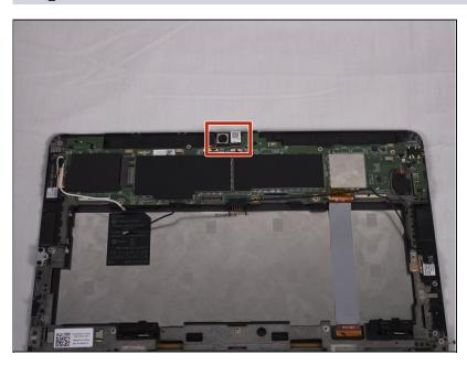
Now turn your attention to the two <u>ZIF</u> connectors at the top. The left ribbon cable connects to the webcam, the right ribbon cable connects to the back camera.
