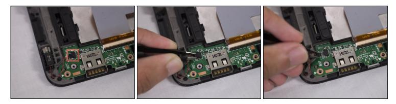
Using a pair of tweezers disconnect the connector from the circuit board
