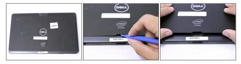
• Turn your device over to the backside. On the notch at the bottom portion of the tablet, use your fingers to lift up the back cover.
