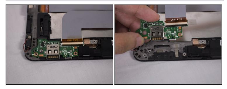
• After disconnecting all the pieces, remove the USB port circuit board with your fingers
