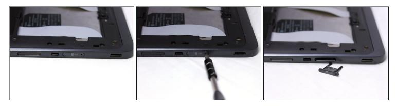
• Use your pin punch driver to push into the hole on the sim card, then pull out the sim tray.
