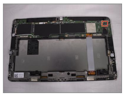
Now you must disconnect the small battery wire located here on the device.
