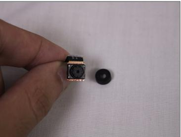
(i) Take caution when removing the front camera with the rubber cover. The cover can easily fall off from any slight movement.
