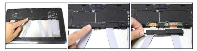
• Slide the cover on the two middle ribbon cables out to remove it. It should uncover the orange cable connectors.
