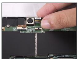
• To remove the right ribbon cable, use the pointy end of your spudger to flip the black <u>ZIF</u> lock upwards. Then pull the ribbon cable rearwards to disconnect it.
