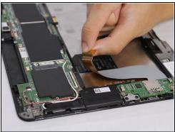
• Wedge the tip of the plastic spudger in between the ZIF connector lock and flip up the lock. Pull the ribbon cable out.
