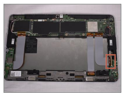
You must then remove the ribbon cable connected to the USB port located here.
