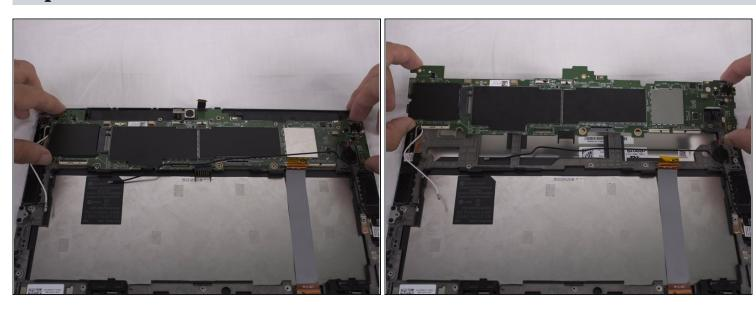
• Finally the motherboard can be lifted out by hand.
