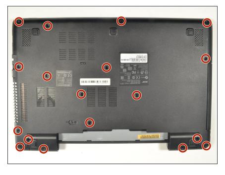
Using a #0 Phillips screwdriver, remove a total of eighteen identical 8mm Phillips screws and set them aside.
