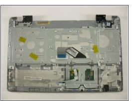
Once all three ribbon cables are disconnected, lift off the top cover with the keyboard and touchpad.
