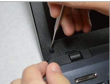
Carefully pry the two rubber covers at the bottom of the screen off with a metal sprudger.
