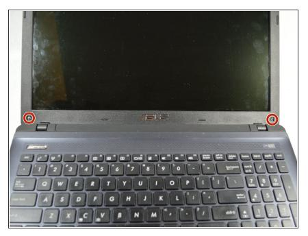
Remove the two 1.84 mm Phillips head screws at the bottom of the screen using PH00 screw driver.
