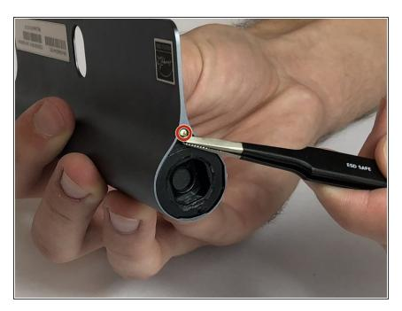
With the hinge removed, locate the end with no wires coming out. Peel back the black screw cover with a pair of tweezers and remove the 3mm screw with a PH00 screwdriver.
