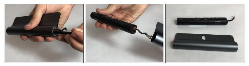
• Begin pushing the battery out using a plastic spudger at the wired end.
