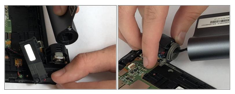
• Begin removing the entire hinge assembly by lifting it out, starting at the end where the lock is located. Carefully feed the wires through the hinge mount with your fingers as you pull the hinge assembly free.
