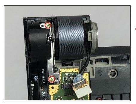
Locate the silver camera mounting bracket between the power button and the camera housing. Remove the two 3mm screws on the camera mounting bracket using a PH00 screwdriver.
