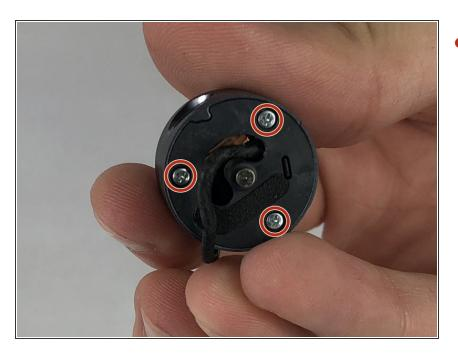
Remove the three 5mm screws holding together the camera housing using a PH00 screwdriver.
