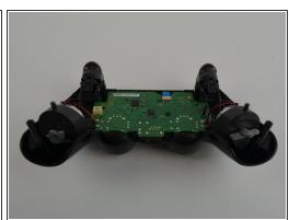
Unhook the battery case from the motherboard, and pull it off.
