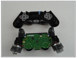
Pull out the second ribbon cable to separate the inner workings from the top of the outer shell.
