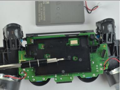
Remove the 6.43mm screw connecting the motherboard to the inner workings of the controller, using a Phillips-Head screwdriver.
