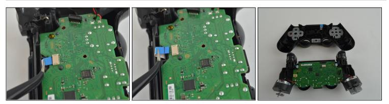
• Pull out the second CPU ribbon to separate the inner workings from the top of the outer shell.
