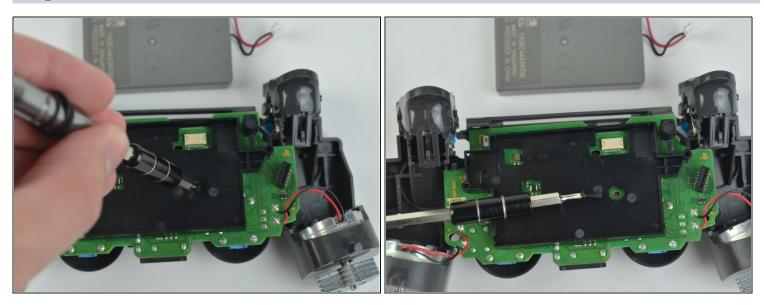
• Remove the 6.43mm screw connecting the motherboard to the inner workings of the controller, using a Phillips-Head screwdriver.
