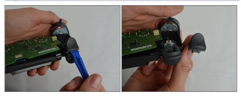
• Insert the plastic opening tool into the space created when the button is pressed down. Make sure the tool is situated directly in the center of the space, before attempting to pry the button out.
