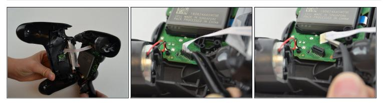
• Pull the ribbon cable out of the motherboard port to fully separate the two halves, using a pair of <u>tweezers</u>.
