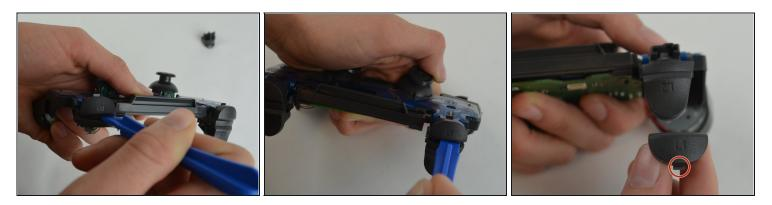
• Pry the button from the controller using the plastic opening tool. Slide the tool between the buttons. There will be a tab you can push in to remove the button.
