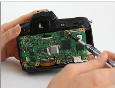
• Use a Phillips #00 screwdriver to unscrew the 2.3 mm screw.
