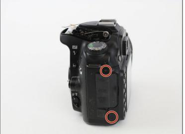
• Using a Phillips #00 screwdriver, remove the four 6.2 mm screws from the left and right sides of the outer cover.
